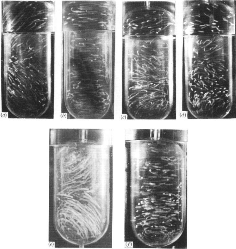
FIGURE 10. Photographs of the change in the nature of the unstable disturbances for L/R = 6 : (a) f = 0.1 , (b) f = 0 , (c) f = -0.06 , (d) f = -0.12 ; for L/R = 4 : (e) f = 0 , (f) f = 0.1 .
